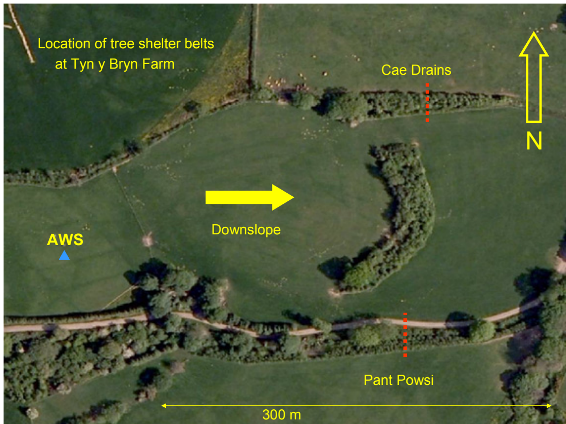
Figure 3.3. Aerial photograph of the tree planted hillslope at Tyn y Bryn farm, showing the main instrumentation for this study; AWS – automatic weather station and its associated rain gauge (blue triangle); dotted lines show siting of instrument transects.
