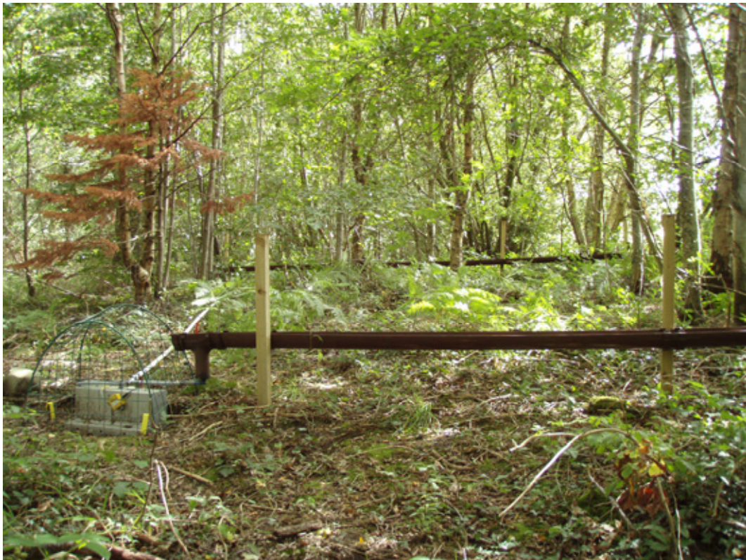
Figure 3.6 Photograph of trough style throughfall collectors within the tree shelter belts showing tipping bucket gauge (foreground, left-hand side).
