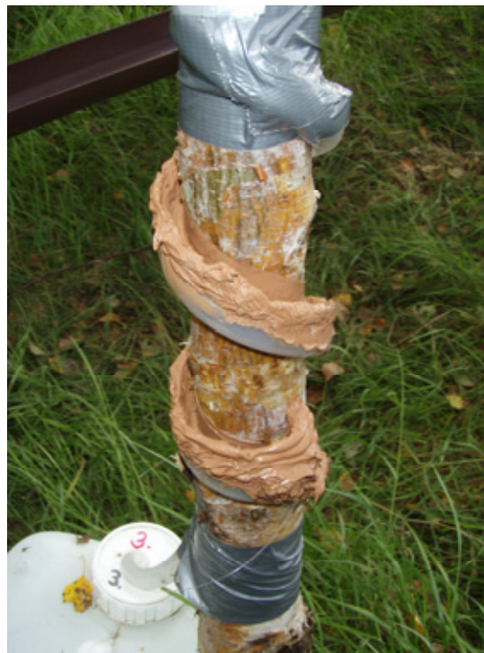
Figure 3.7. Stemflow collector attached to a silver birch
